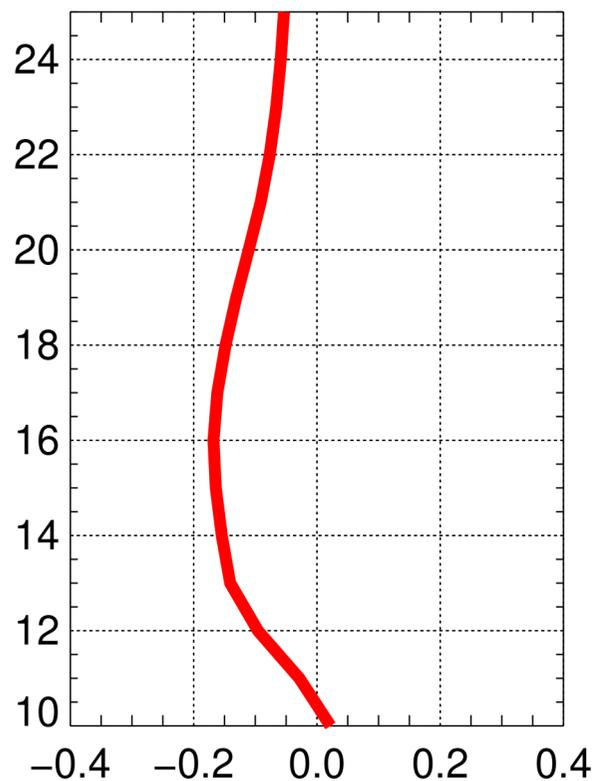
Mean relative difference between retrievals for ACE-FTS collocations (10) neglecting and accounting for stratospheric aerosols
