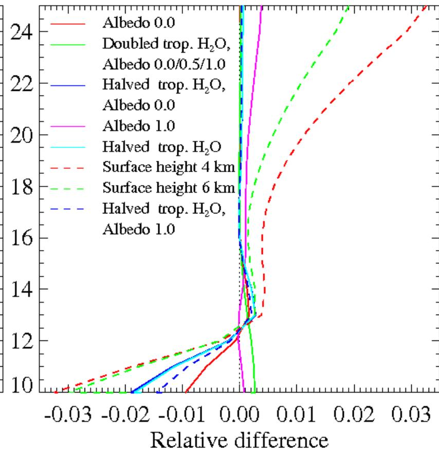
Simulations were performed for surface albedo of 0.5 and surface elevation of 2.2 km
